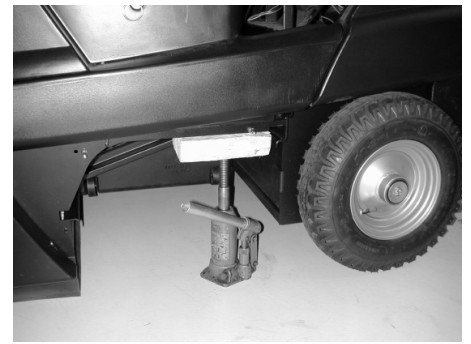
Intake point for the jack (rear wheels)
