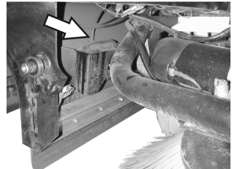
Hose connection at the vacuum pressure socket of the side brush lowering system
